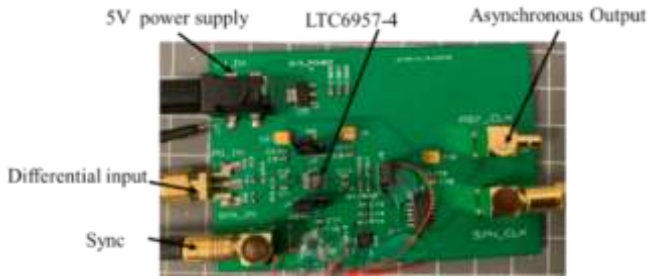
Fig.7. The custom-designed PCB for the ADC clock driver
