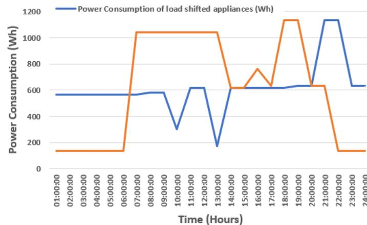
Figure 11. 24-h winter power consumption graph for load shifted with and without an HEMS.
