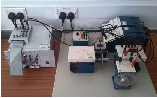
Fig. 6. Networked servo motor system.
