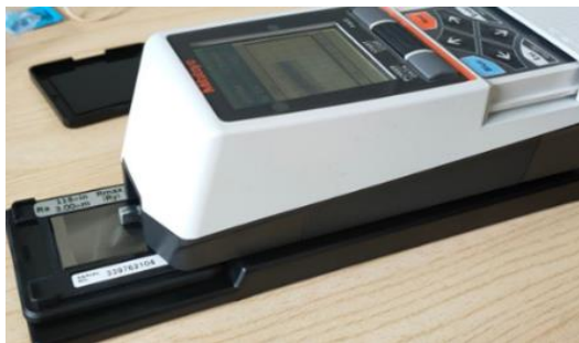
Fig 4. Mitutoyo SurfTest SJ-210 with 3.00 \mu\text{m} Ra calibration reference
