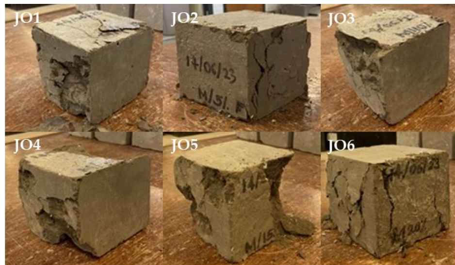
Figure 8. Performance of concrete cube specimens subjected to freeze and thaw cycles after Compressive Strength test.
