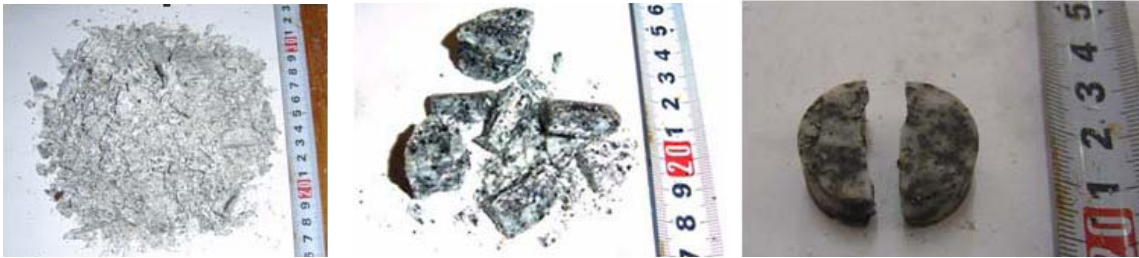
(a) d=75\text{mm} , \dot{\epsilon} = 98.23\text{s}^{-1} (b) d=36\text{mm} , \dot{\epsilon} = 99.75\text{s}^{-1} (c) d=22\text{mm} , \dot{\epsilon} = 164.38\text{s}^{-1} Fig.3 Fragmentation of granite specimens with different sizes under different strain-rates [21]
