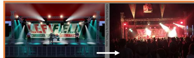
A common industry use of WYSIWYG (left), to show touring Lighting Designers the design concept for a stage lighting rig, in this case: Leftfield Stage, Glastonbury 2019 (right).
