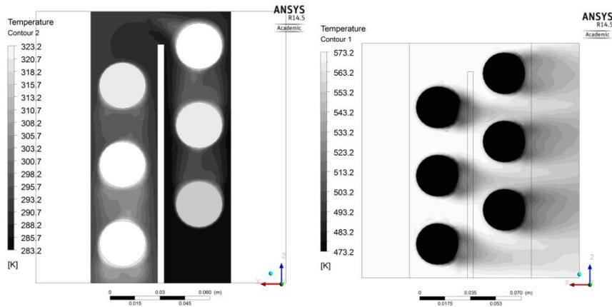
Figure 5: Visualisation of CFD results. Condenser (left) and evaporator (right) ( $T_{h,in} = 300\text{ °C}$   $\dot{m}_{h,in} = 0.2\text{ m/s}$ ,  $T_{c,in} = 10\text{ °C}$   $\dot{m}_{c,in} = 0.07\text{ m/s}$ ). Conversion Kelvin – Centigrade:  $10\text{ °C}$  (283 K),  $50\text{ °C}$  (323.2 K);  $200\text{ °C}$  (473.2 K),  $300\text{ °C}$  (573.2 K).
