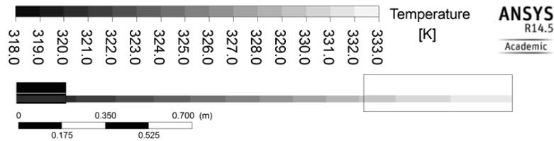
Figure 4: Temperature profile of the heat pipe ( $T_{h,in} = 300\text{ °C}$   $\dot{m}_{h,in} = 0.2\text{ m/s}$ ,  $T_{c,in} = 10\text{ °C}$   $\dot{m}_{c,in} = 0.07\text{ m/s}$ ).
