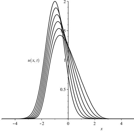
Fig. 2. The first thirty terms in the series solution from equation (6) are used to produce distributions of  $u(x, t)$  at times  $t = 0, 0.2, 0.4, 0.6, 0.8$  and  $1.0$  where  $\epsilon = 0.5$ . These distributions propagate from left to right as  $t$  increases (cf. numerical solutions in Fig. 1).
