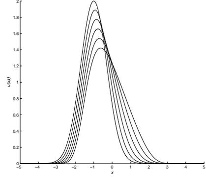
Fig. 1. Equation (3) is solved numerically with initial data  $u(x, 0) = 2e^{-(x+1)^2}$  and  $c(x) = 1 + \epsilon \sin x$  where  $\epsilon = 0.5$ . The solutions for  $u(x, t)$  are shown at times  $t = 0, 0.2, 0.4, 0.6, 0.8$  and  $1.0$ . The distributions propagate from left to right as  $t$  increases.
