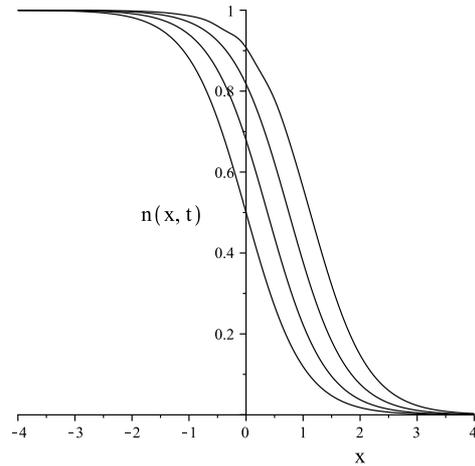
Fig. 4. The first twelve terms in the series solution from equation (18) are used to produce distributions of  $n(x, t)$  at times  $t = 0, 0.25, 0.5$  and  $0.75$ . All model parameters are set to unity.
